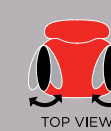
R Arm Rotation Rotate armcap to support your forearm in various positions. Reduces muscular effort in neck and shoulders, minimizing risk of pain.
