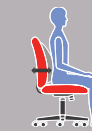
V Lumbar Depth Adjustment Increase or decrease curvature of the back to match the profile of your lower back. Enhances comfort and support in the lower lumbar area.
