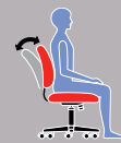
G Back Angle Adjust to change the angle of your torso in relation to your thighs. Helps reduce disc pressure and relaxes your back muscles.
