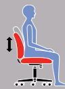
D Back Height Raise or lower to position lumbar support in your lumbar area. Reduces likelihood of back pain.
