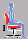
C Seat Height Raise or lower to allow your feet to rest flat on the floor. Avoids pressure under your thighs, easing blood flow.
