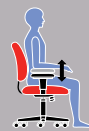
H Arm Height Raise or lower to support your forearms. Reduces muscular effort in neck and shoulders, minimizing risk of pain.
