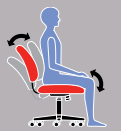
A Tilt Tension Increase or decrease to match body weight. Allows you to rock comfortably, without heavy pushing, reducing muscle fatigue.
