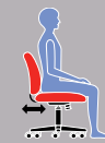
E Seat Depth Change the depth of the seat to accommodate the length of your thighs. Keeps your back in contact with the backrest while avoiding pressure behind your knees.
